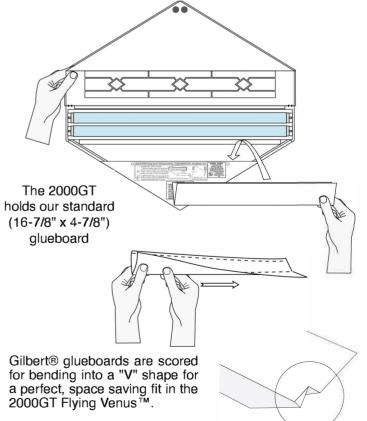
If necessary, to prevent lamp heated glue from oozing out the end of the "V", bend 1/2" up at each end (forming a tray to contain glue).
