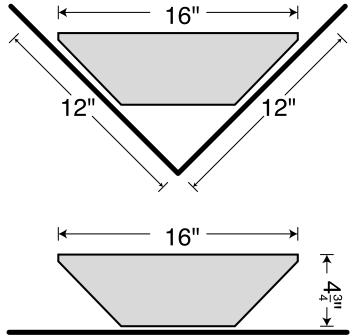
The Junior™, mounts like the rest of the 601 series of traps, in a corner or flat against the wall.
